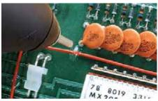
Product assembly with a slim profile to help operators apply adhesive more accurately.
